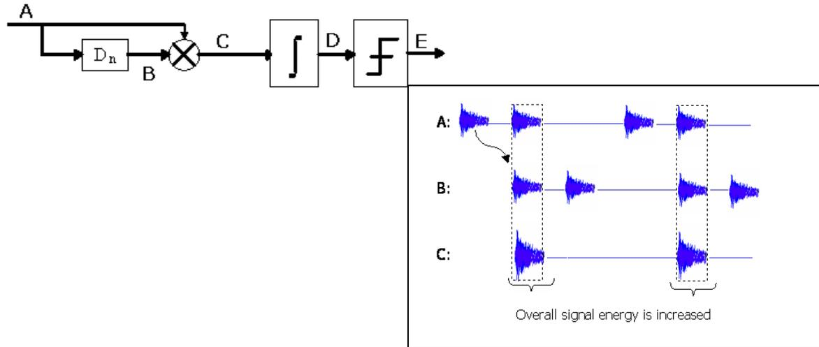
**Figure 2: (Left) Block diagram of a multipulse receiver (similar to Fig.2). D<sub>n</sub> is the delay between the transmitted pulses. (Right) Signal representation of multipulse receiver in multipath channels. Due to passing through the same channel, the signal energy for correlation is stronger.**
