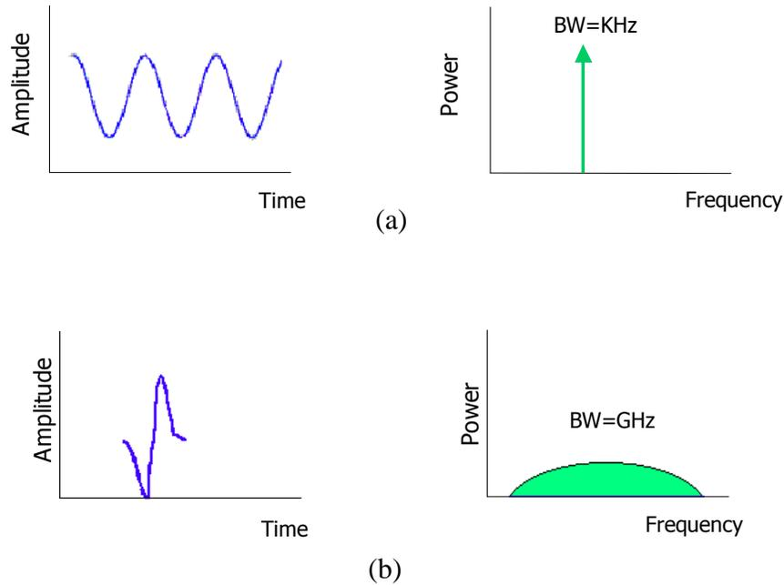
**Figure 1. (a) Conventional narrowband communications send long continuous waveforms and generate very narrow frequencies. (b) UWB communications send extremely narrow pulses and generate very wide frequencies.**
